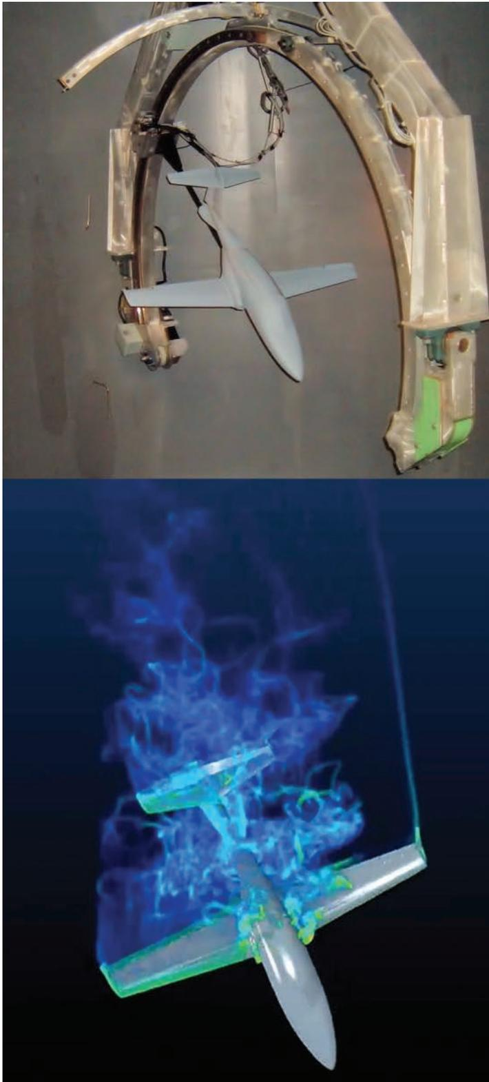
Figure 10: Tunnel Model (Top) - Spin Simulation on XFlow (Bottom)
