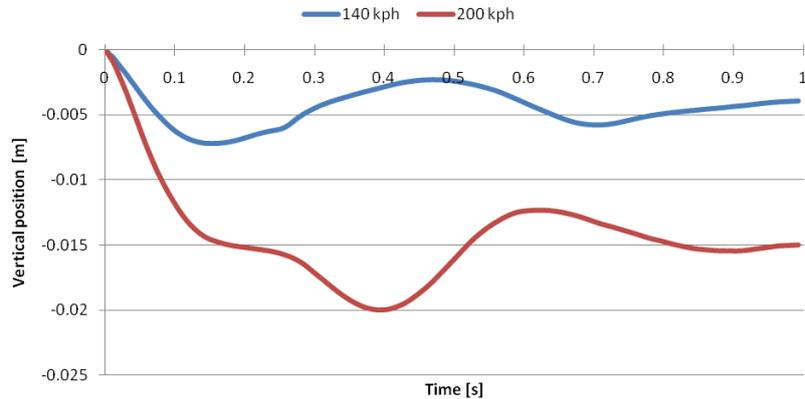
a) Vertical displacement at CoG (in meters)
